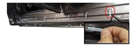
Step 4: Take No.9 splicing nut, put in the snaps hole which locate in 2-9 place, ensure splicing tail is straight down and fasten, total 8pcs;
