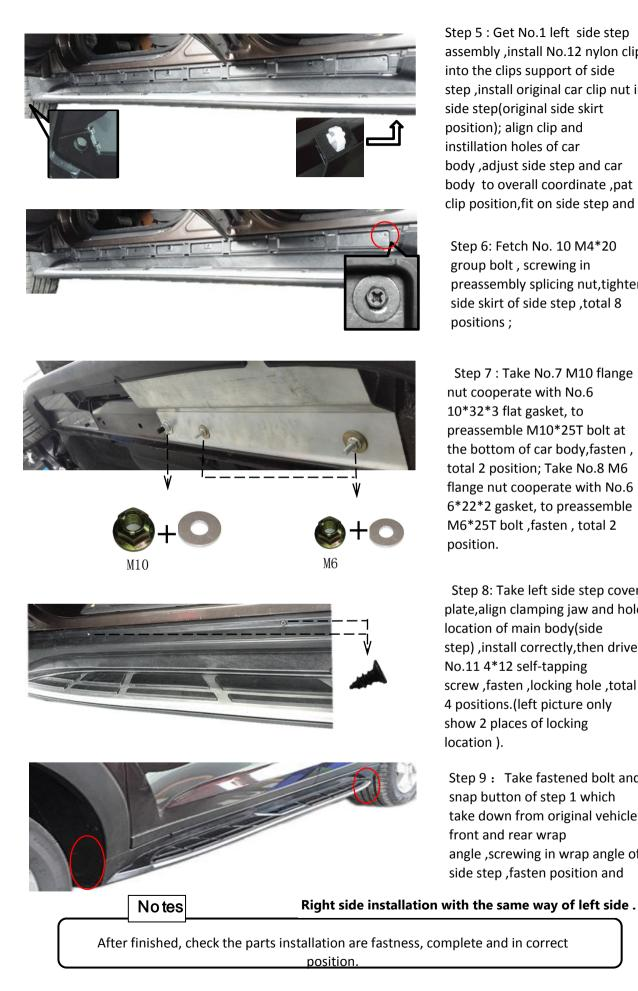
Step 5 : Get No.1 left side step assembly, install No.12 nylon clips into the clips support of side step, install original car clip nut in side step(original side skirt position); align clip and instillation holes of car body, adjust side step and car body to overall coordinate ,pat clip position, fit on side step and
