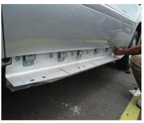
3. Now take the step cover and place it on the core, align holes (especially the middle one). Also align the clips with the tabs in order for them to snap in. Replace the push tabs at the rear and front wheel arch linings making sure everything is aligned. You can either use the newly supplied pins or reuse the original Mercedes ones. Finally insert the 5 rubber pins on top of the running board aligning them so that you will be able to see them underneath the car.
