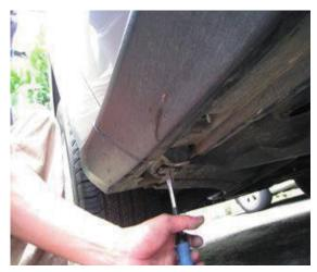
2. Now you have to unscrew the metal hex nuts on the plastic core frames on the side. Then you take the replacement side step and separate the step cover from the aluminium/plastic core (depending on the set). You replace the plastic frames with the large core from the received set. You just slide it onto the studs (it is easier with doors open). By hand screw in the nuts with washers and once all are in place tighten them. Be careful not to brake the studs of.
