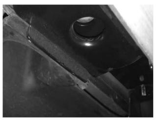
5. On the underside plastic part of the running board you will find smaller holes, this is where the plugs from the top should come out. You secure them with the black washer nut. The whole plastic bit has to go under the metal ridge. Just pull it back firmly and slide it under. Tighten all nuts and bolts and you are done.
