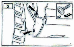
Step 1. After removing the screws you open up the doors and try to pull out the plastic sill from underneath the car by pushing it down and out (beginning from the rear and pulling along to the front). While removing the sill you will see yellow popper clips underneath the sill, on the car body. Once all clips are separated from their counterparts (those will remain on the sill) you have to pull the sill out to the back, so that it clips out of the front.
