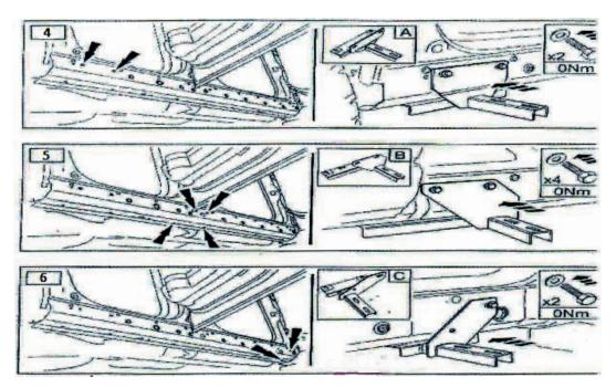
Step 5. At this point you will have to cut out holes in the plastic sill trim for the brackets to fit in. They should be originally marked out by the manufacturer. You can also place the sill next to the mounted brackets to double check the placement of the holes.
