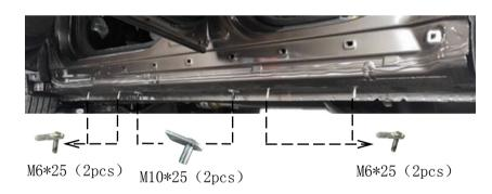
Step 2: Take No.3 M10\*25T bolts, put in the second and third water pore, total 2 pcs; Step 3: Take NO.4 M6\*25T bolts, put in the small square hole which between the first and second water pores, and the hole which between the third and fourth circular hole, total 4 pcs.
