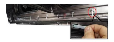
Step 4: Take No.9 splicing nut, put in the snaps hole which locate in 2-9 place, ensure splicing tail is straight down and fasten, total 8pcs;
