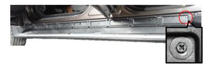
Step 5 : Get No.1 left side step assembly ,install No.12 nylon clips into the clips support of side step ,install original car clip nut in side step(original side skirt position); align clip and instillation holes of car body ,adjust side step and car body to overall coordinate ,pat clip position,fit on side step and
