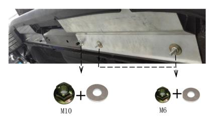
Step 7: Take No.7 M10 flange nut cooperate with No.6 10\*32\*3 flat gasket, to preassemble M10\*25T bolt at the bottom of car body,fasten, total 2 position; Take No.8 M6 flange nut cooperate with No.6 6\*22\*2 gasket, to preassemble M6\*25T bolt,fasten, total 2 position.
