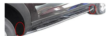
Step 9: Take fastened bolt and snap button of step 1 which take down from original vehicle front and rear wrap angle ,screwing in wrap angle of side step ,fasten position and
