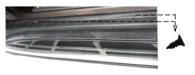
Step 8: Take left side step cover plate, align clamping jaw and hole location of main body(side step), install correctly, then drive No.11 4\*12 self-tapping screw, fasten, locking hole, total 4 positions. (left picture only show 2 places of locking location).
