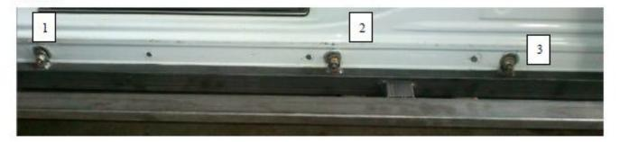
Step 5: Install the buckle in white color to the running board. And then install the running board to the fitted brackets, align and level them to proper position, and press it to make all the buckles fitted. Fasten all the hardware to finish installation.
